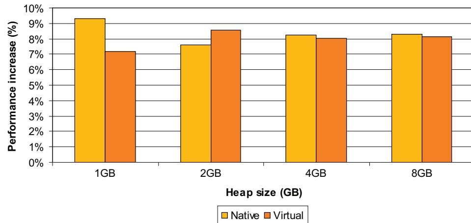
Figures 1 and 2 show the SPECjbb2005 results for Red Hat Enterprise Linux 4 Advanced Server and Windows Server 2003, respectively. The Java virtual machine heap size varies from 1GB to 8GB, in order to represent different working set sizes.
