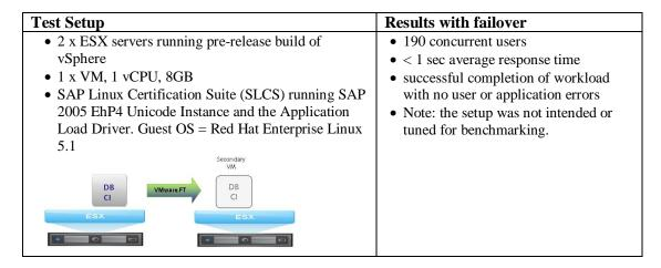
Figure 6. LinuxLab@SAP Workshop Results - VMware FT Test with VM running DB + CI
