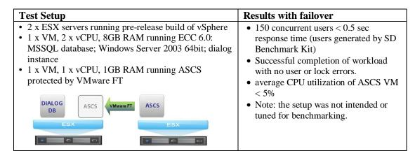
Figure 4. Lab Results - VMware FT Test with VM running ASCS
